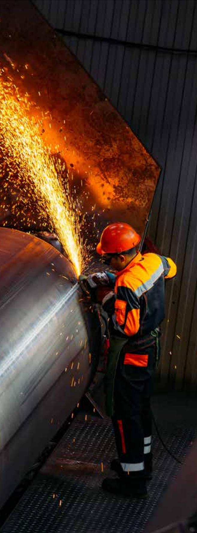
EXITFLEX grinding discs are renowned for maximum stock removal in a short span of time. EXITFLEX grinding wheels are used in all major surface grinding applications, as well as for edge beveling and burr removal.
